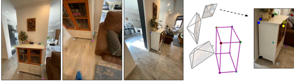
Figure 3: Bundle adjustment can be extended to a global 3D object track. Each observation of a track is characterized by an image and particular 3D box detection from CuTR. Since these individual 3D boxes (shown as thin, white boxes) are usually aligned well with the RGB image, they can be used to enforce a reprojection cost function by comparing the projected corners of these detections to the projected corners of the object track’s representative 3D box. The point tracks established in Section 3.3 (shown in 8 colors) allow us to map the corners of these individual 3D boxes to the corners of the track’s global 3D box. In the rightmost pane, we show an initial mismatch of the projected corners from the individual detection (brighter color) and the object track (darker color) that may be minimized by optimizing the track’s 3D box parameters.
