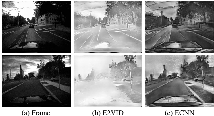
Figure 4: Challenging scenes from the MVSEC dataset (Zhu et al., 2018a). Depicted are (a) the conventional frame images, (b) failed predictions of E2VID (Rebecq et al., 2019b), and (c) the predictions of ECNN (Stoffregen et al., 2020). Since ECNN shares the architecture with E2VID but was trained on augmented data to reduce the sim-to-real gap, the predictions are notably more robust.
