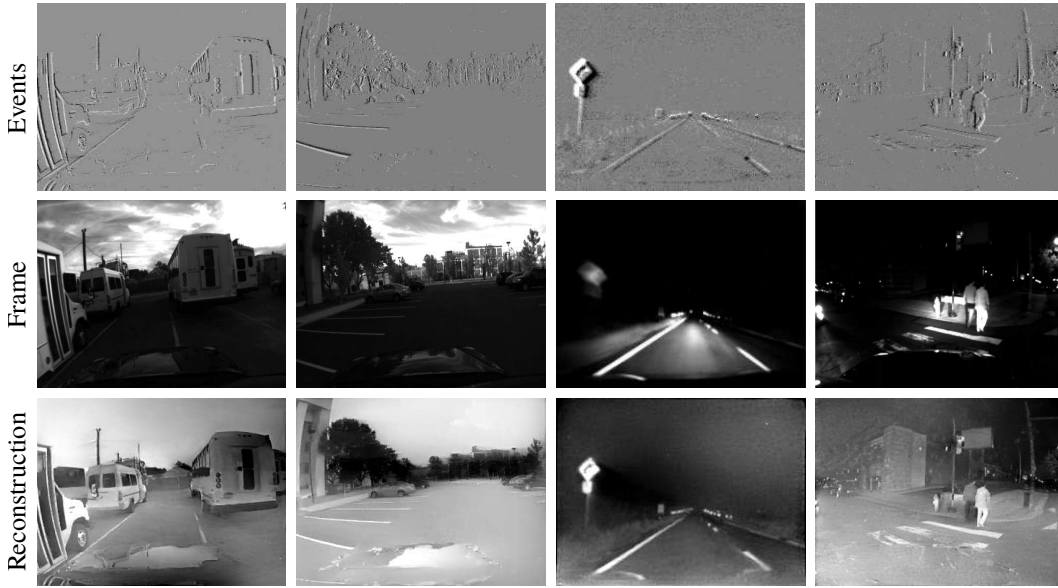
Figure 2: Image reconstructions of E2VID from Rebecq et al. (2019b) in driving scenarios under challenging lighting conditions. The first row shows event frames, while the second row shows images from a regular camera. The reconstructions of E2VID in the third row can capture the scene in a high dynamic range and without motion blur.
