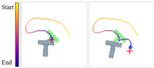
Figure 7: Non-Smooth Trajectory Generation. A Push-T trajectory generated by our Neural SDE, showcasing its ability to handle drastic changes in direction.
