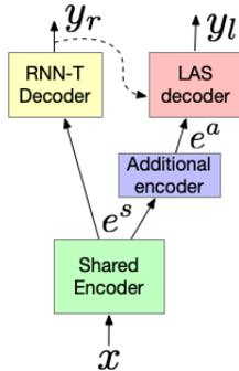
Fig. 1: Two-Pass Architecture
