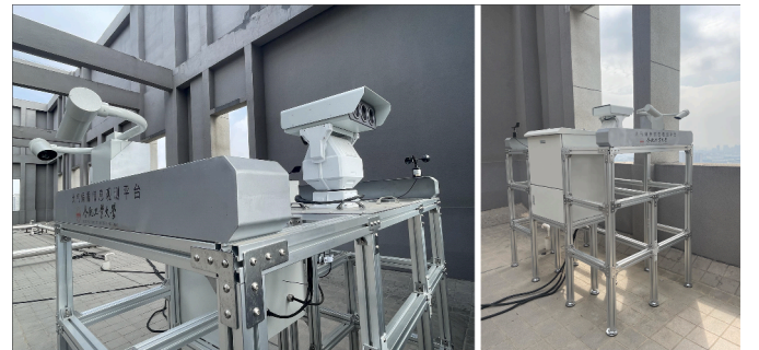
Fig. 2. Our fixed atmospheric polarization information observation platform, the UAV atmospheric polarization information observation platform can be seen in Section 4.1. We conducted extensive field observation experiments under foggy, hazy and other weather conditions, and obtained multi-target polarization data under various meteorological conditions.
