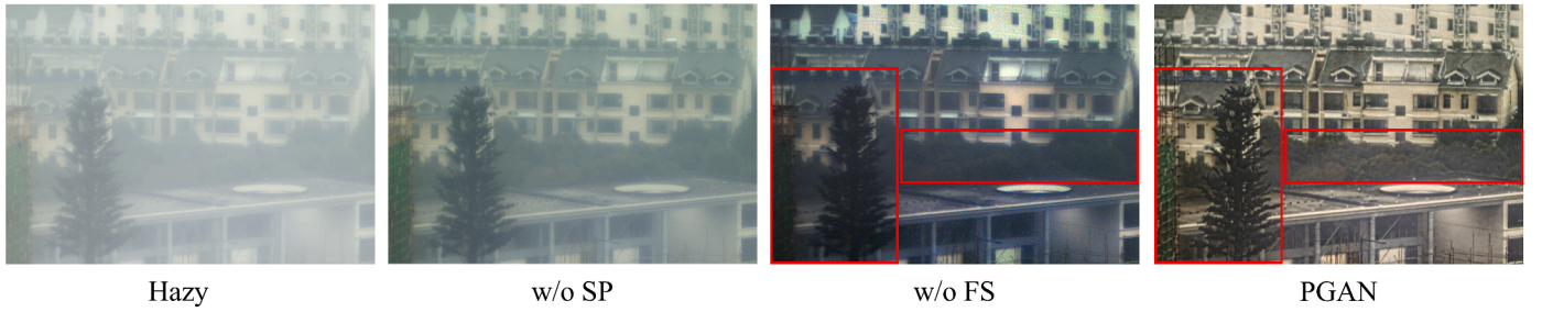
Fig. 10. Qualitative results of the ablation experiment. “w/o SP” means removing the Stokes calculation module of PGAN-A and replacing the input with the original hazy image. “w/o FS” represents for removing the frequency decomposition module of discriminator and the pseudo airlight coefficient supervision loss.
