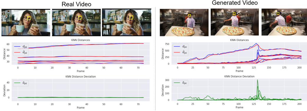
Figure 5: Deviation of neighbor tracks on real video vs generated video with object distortions. Blue plot: Distance between a nearest neighbor and a candidate point. Red plot: Moving average of blue. Green plot: the deviation between blue and red.
