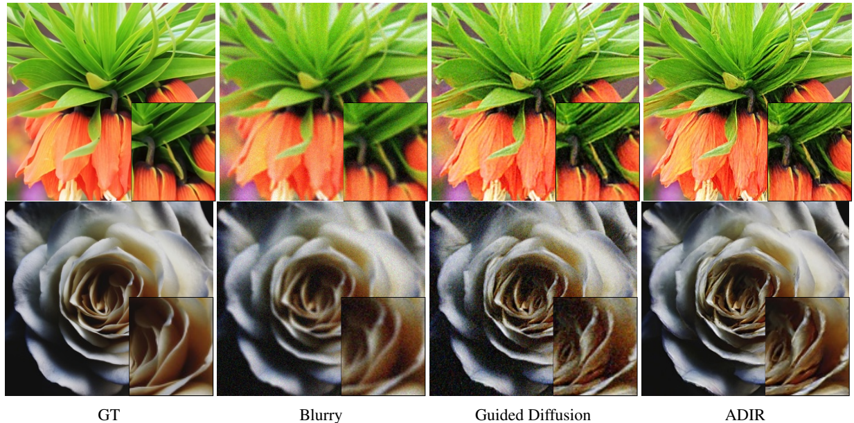
Figure 5: Image deblurring using Guided Diffusion approach from section 3.2 and ADIR, using the unconditional model from (Dhariwal & Nichol, 2021). The degradation is performed using 5 \times 5 uniform blur filter with 10 levels of additive Gaussian noise. Note the better quality of our method.
