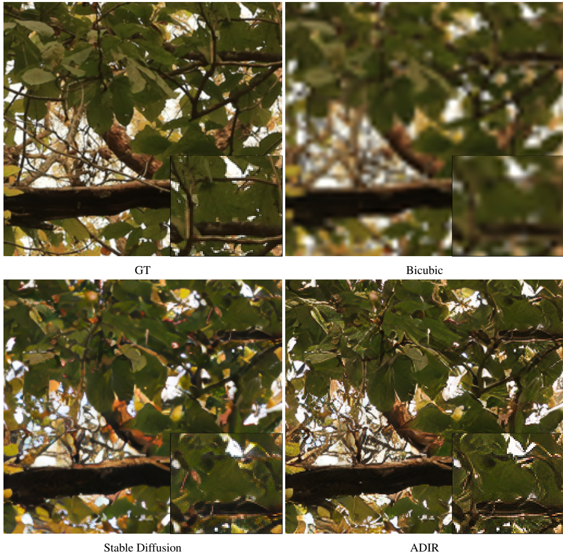
Figure 11: Comparison of super resolution ( 256^2 \rightarrow 1024^2 ) results of Stable Diffusion (Rombach et al., 2022) and our method (ADIR), using the unconditional model from (Rombach et al., 2022). As can be seen from the images, our method outperforms guided diffusion in both sharpness and reconstruction details.
