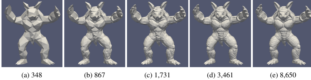
Figure 9: Visualization of different mesh resolutions. The captions denote the number of vertices.
