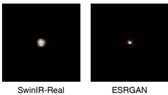
Figure 10. The impulse response of SwinIR-Real (Liang et al., 2021) and ESRGAN (Wang et al., 2018) is not an obvious sinc function.
