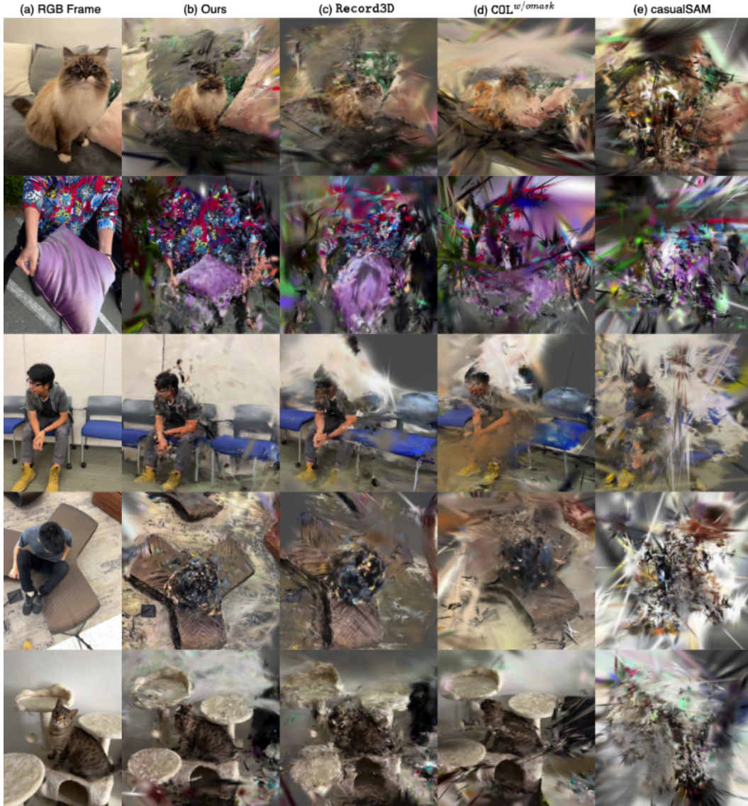
Figure 19: Optimized 3D Gaussian Fields on iPhone [7] - Part 1. Our reconstructed 3D Gaussian Fields are more geometrically accurate compared to the ones of other RGB-only supervised methods, which demonstrates our camera estimates are more accurate. Besides, our performance is comparable with, or even better than, the ones of the LiDAR-based Record3D app.
