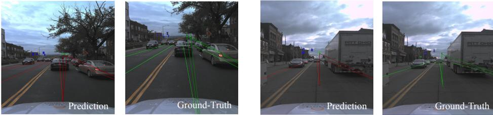
Figure 4: **Traffic detection and lane-traffic topology from TopoMLP.** Our method can detect the traffic elements in the front view and associate them with lanes. The **green** represents GT, while the **red** means our prediction. Traffic predictions are grounded by different colors in terms of category.
