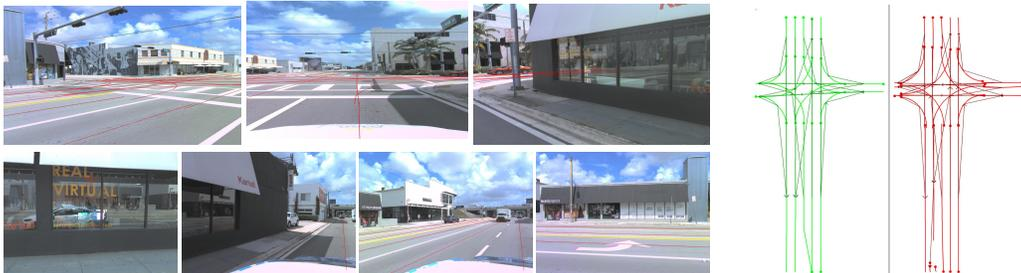
Figure 3: **Qualitative results for lane detection and lane-lane topology of TopoMLP.** Given the multi-view images, our method can predict the most lanes and connect them correctly under various challenges, like occluded lanes and complicated intersections. The **green** lanes are ground-truth and the **red** lanes are predictions, which are projected into images and BEV map.
