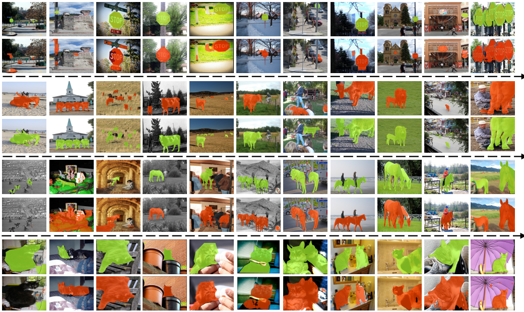
Figure 7: Visualization of online few-shot segmentation performance on COCO. Ground-truths are masked in green and predictions are masked in red. The length of sequence is set as T = 11 , and 0-shot to 10-shot results are reported. The input sequence exhibits large sample diversity, our model shows superior capacity in tackling this problem.
