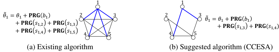
Figure 1: Conventional secure aggregation (SA) (Bonawitz et al., 2017) versus the suggested communication-computation efficient secure aggregation (CCESA). Via selective secret sharing across only a subset of client pairs, the proposed algorithm reduces the communication cost (for exchanging public keys and secret shares among clients) and computational cost (for generating secret shares and pseudo-random values, and performing key agreements), compared to the existing fully-shared method. CCESA still maintains virtually the same levels of reliability and privacy, as proven by the theoretic analysis of Section 4.
