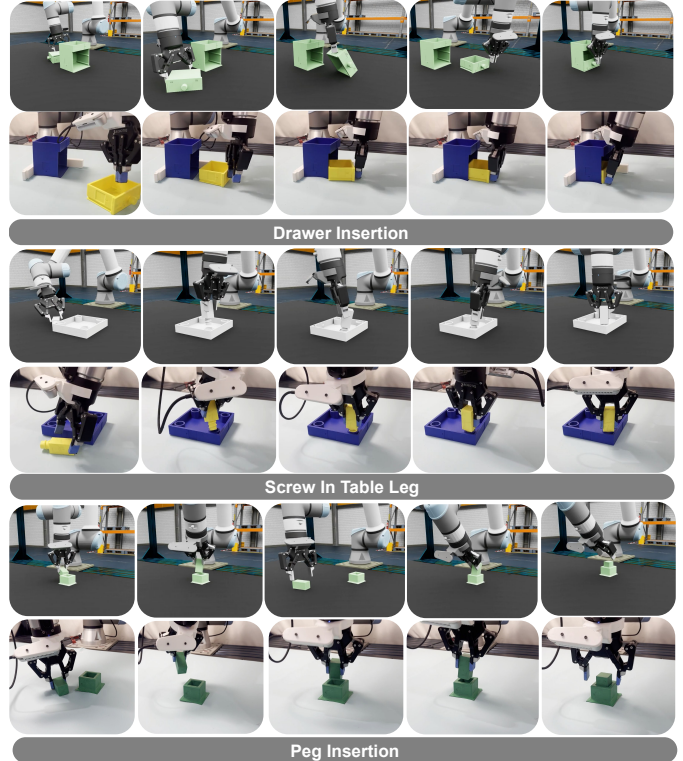
Fig. 1. OmniReset uses diverse simulator resets and large-scale RL to solve contact-rich, long-horizon tasks. Policies are distilled to RGB inputs and transferred to the real world zero-shot.
