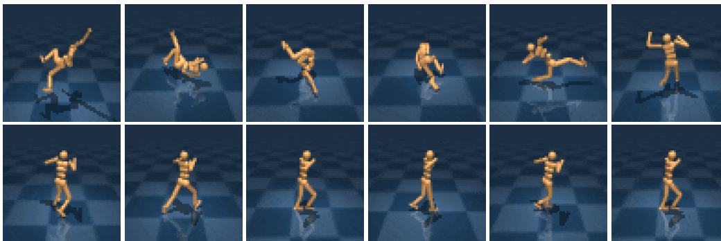
Figure A1: Behavior learned by DreamerV2 on the Humanoid Walk task from pixel inputs only. The task is provided by the DeepMind Control Suite and uses a continuous action space with 21 dimensions. The frames show the agent inputs.
