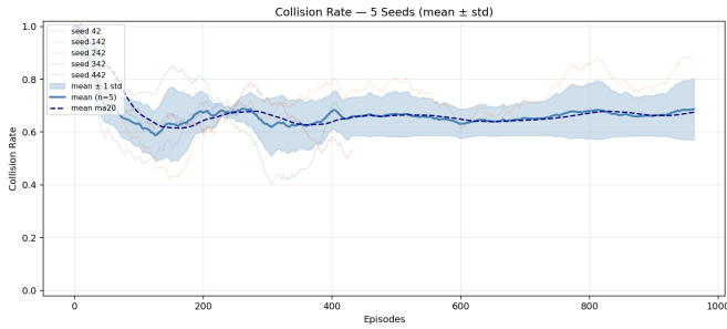
Fig. 10. Per-episode collision rate over training (mean \pm 1 SD across five seeds). Mean falls from \sim 1.0 to 0.65 \pm 0.13 in the final episodes; lower is better.
