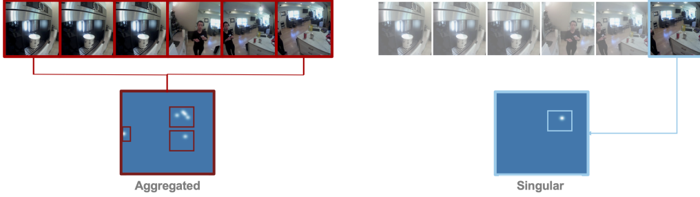
Figure 8: Illustration of singular and aggregated gaze heatmaps. For the singular gaze heatmap, only the gaze point associated with the final heatmap is utilized. On the other hand, for the aggregated gaze heatmap, gaze points over an interval \delta = 200ms are collected to form the aggregated heatmap.
