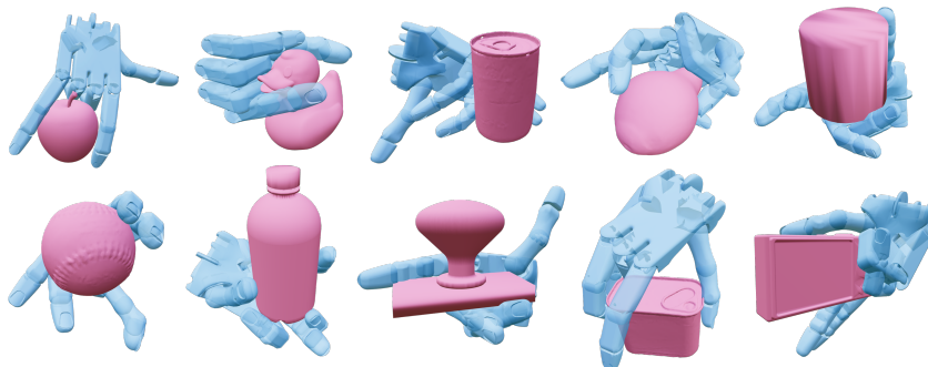
Figure 11: Grasp examples filtered out from the dataset that would otherwise be deemed successful under static metric.
