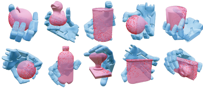
Figure 8: Grasp examples with partial object point clouds. Red points show the observed portion.
