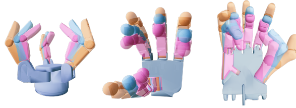
Figure 10: Visualization of the grasp controller’s effect: blue indicates the predicted grasp pose, orange represents q_{\text{outer}} , and pink represents q_{\text{inner}} .
