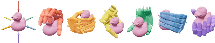
Figure 6: Diverse and pose-controllable grasp generation. The arrow refers to the input palm orientation. Arrows and hands of the same color represent corresponding input-output pairs.
