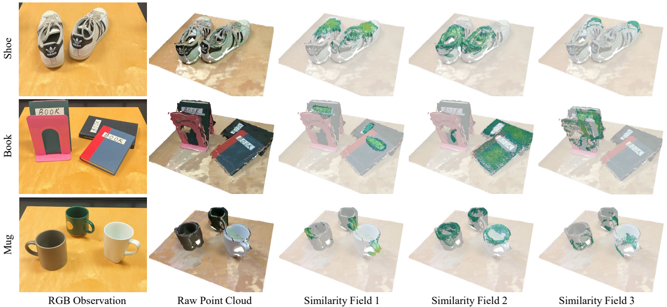
Fig. 6: Similarity Fields Visualization. We visualize 3D similarity fields in the scene where multiple instances from the same category are presented. It is observed that the similarity fields exhibit similar patterns for different instances. For example, all book titles are highlighted, regardless of whether they are different books in different poses. Furthermore, these highlighted areas represent semantically meaningful parts and are important for various tasks, such as shoelaces, shoe heads, book stands, mug handles, and so on.
