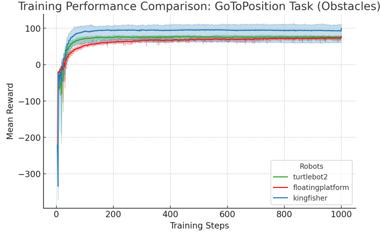
Figure 7: Training performance on GoToPosition with static obstacles for three robots. Curves show mean and std reward over 10 seeds. All robots learn stable obstacle-avoiding behaviors; the final-50-step mean rewards are Kingfisher \approx 93.4 , Turtlebot2 \approx 75.4 , and FloatingPlatform \approx 73.0 .
