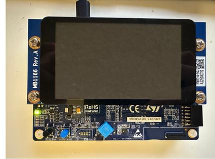
**Fig. 8: The STM32H747 device for model deployment.**
