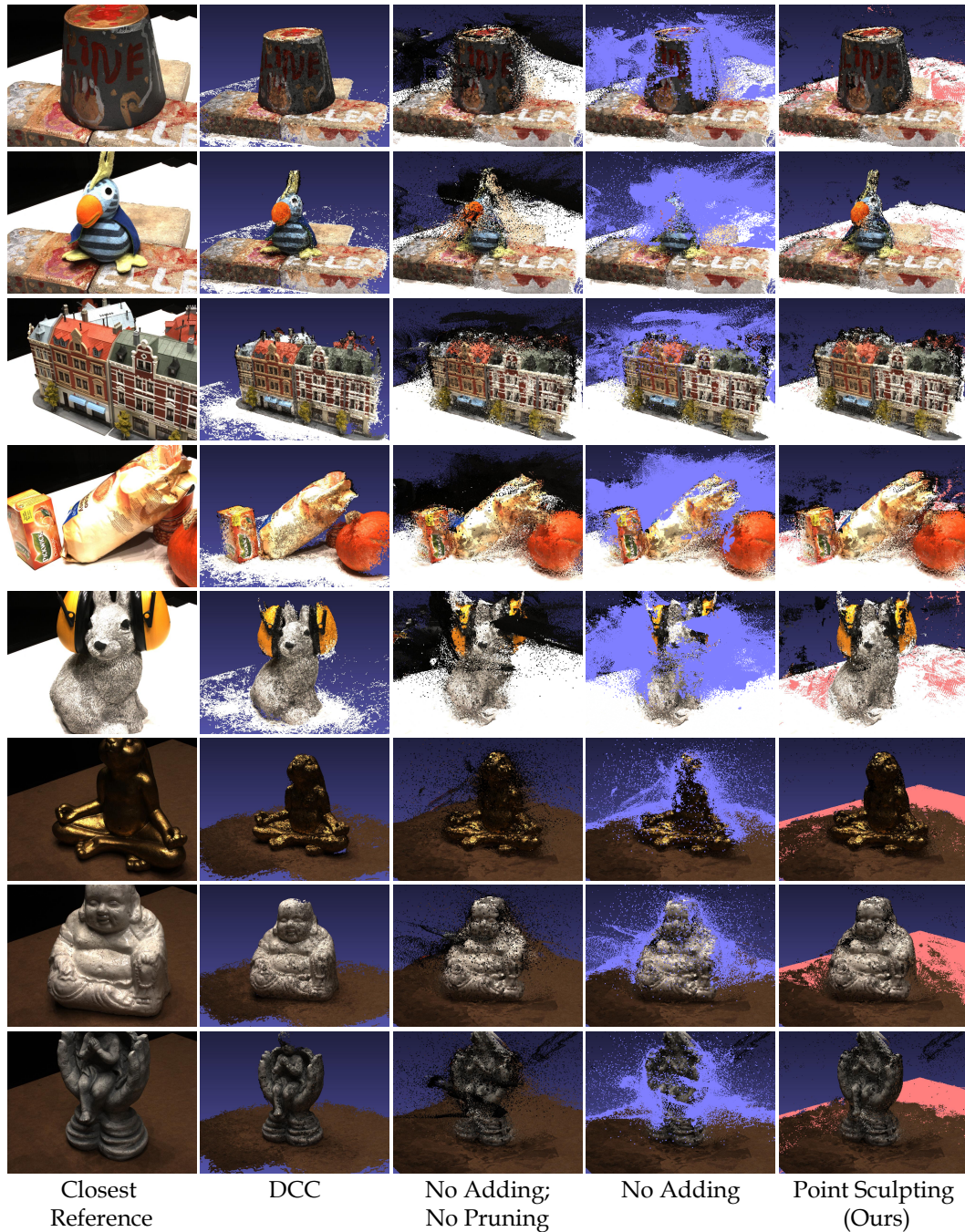
Figure 11: Qualitative comparison of different point cloud refinement algorithms. Compared to the initial point cloud (“No Adding; No Pruning”), our point sculpting method removes the outliers (the blue ones in the “No Adding” column), and adds new points (the red ones) that further fill the missing areas. Although DCC (Yan et al., 2020) provides point clouds with higher accuracy in the foreground, the completeness is much worse than our results. For scenes where the initial point cloud quality is low (e.g., the bottom 3 rows), more points are used to fill the holes. Although the final sculpted point cloud can still contain outliers and small holes, those can be handled by the gradient-based refinement.
