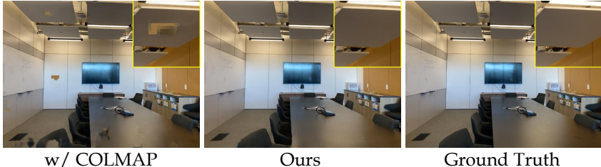
Figure 9: We visually compare the results of using the COLMAP fused point cloud against our proposed MVS finetuning + point sculpting. Our point cloud has higher completeness and thus better visual quality, especially in texture-less areas (e.g., the zoomed-in ceiling region).
