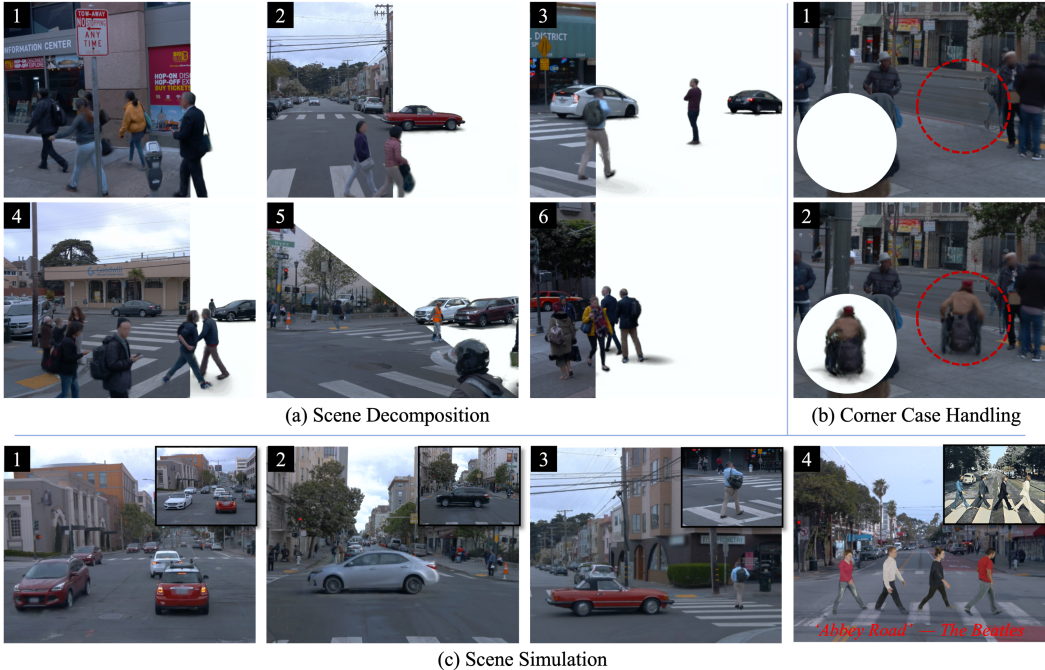
Figure 1: (a) Decomposition of different parts of a scene. (b) Out-of-distribution categories that are overlooked by previous methods can be accurately handled by Omn iRe . (c) Omn iRe enables diverse applications including vehicle editing (c1, c2), human-vehicle interaction (c3), human behavior simulation (c4), etc.
