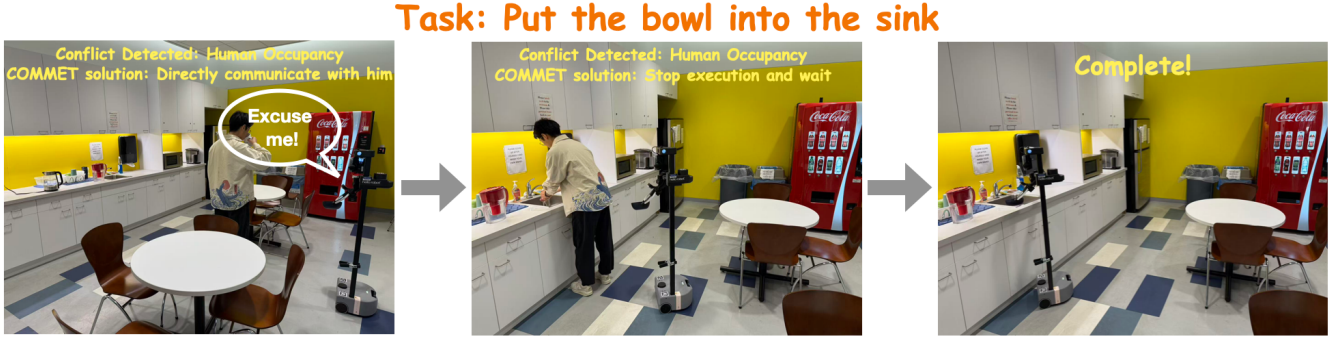
Fig. 4. Real-world Pipeline Example. Suppose the task is to put the bowl into the sink. On the robot's way to the sink, a human is blocking the way. After identifying the conflict type, COMMET reasons based on the user preference data, successfully completing the task.
