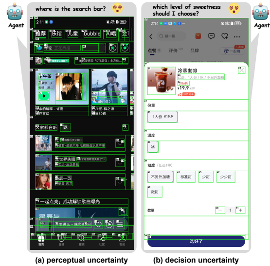
Figure 1: The two major challenges faced by existing GUI Agents: (a) Perceptual uncertainty caused by input redundancy. For example, when searching in a music application, excessive input redundancy prevents the Agent from locating the search box component. (b) Decision uncertainty caused by the lack of interactive mechanisms. For example, the Agent does not know which sweetness level to select for the user when helping with coffee ordering. The input used here is in SoM (Yang et al., 2023) format.
