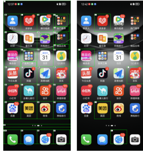
Figure 4: Visualization of SoM outputs before and after using the Component Recommendation Module. Left: original; right: with module. Current goal: “open a shopping app”.
