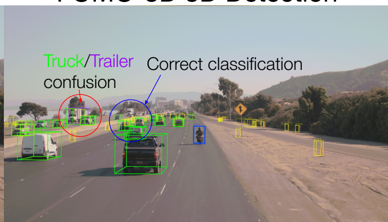
Figure 12: [Highway] Qualitative example #1. Green denotes vehicle. Purple denotes towed object. Blue denotes cyclists. Orange denotes person. Yellow denotes cone. Opacity of the boxes reflects detection confidence (higher confidence corresponds to more solid lines). FP=False Positive. FOMO-3D is able to correct various errors in OWL and LiDAR-only detections, but still mis-classifies a truck as trailer.
