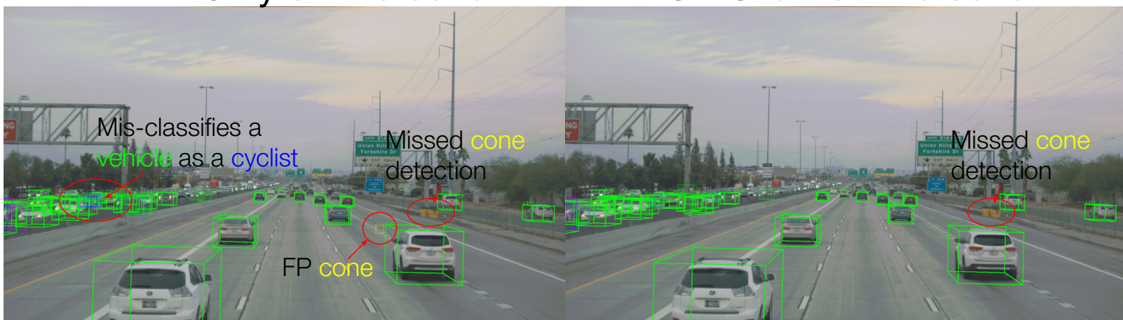
Figure 13: [Highway] Qualitative example #2. Green denotes vehicle. Purple denotes towed object. Blue denotes cyclists. Orange denotes person. Yellow denotes cone. Opacity of the boxes reflects detection confidence (higher confidence corresponds to more solid lines). FP=False Positive. This example shows a very dense traffic scene on the highway. OWL has impressive zero-shot 2D detections, but it also outputs a few false positives. LiDAR-only model mis-classifies a vehicle as a cyclist, and also draws a false positive cone. FOMO-3D is able to correctly classify in most cases without having many false positives. All three detectors miss two cones on the right.
