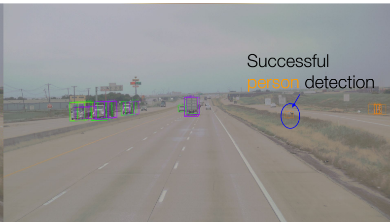
Figure 15: [Highway] Qualitative example #4. Green denotes vehicle. Purple denotes towed object. Blue denotes cyclists. Orange denotes person. Yellow denotes cone. Opacity of the boxes reflects detection confidence (higher confidence corresponds to more solid lines). FP=False Positive. In this example, the LiDAR-only model misses the person on the right, while OWL is able to detect it. With effective multi-modal fusion, FOMO-3D successfully detects the person.
