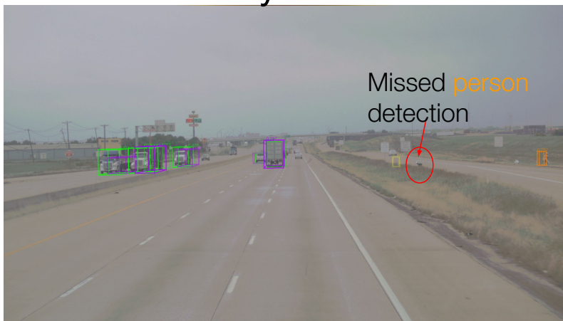
Figure 15: [Highway] Qualitative example #4. Green denotes vehicle. Purple denotes towed object. Blue denotes cyclists. Orange denotes person. Yellow denotes cone. Opacity of the boxes reflects detection confidence (higher confidence corresponds to more solid lines). FP=False Positive. In this example, the LiDAR-only model misses the person on the right, while OWL is able to detect it. With effective multi-modal fusion, FOMO-3D successfully detects the person.
