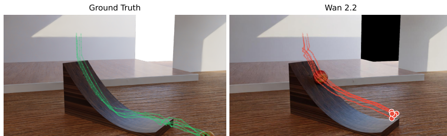
Figure 7: Point tracking visualization on ramp_launch . GT trajectories (green) show correct parabolic motion after ramp exit. Wan 2.2 predictions (red) diverge during projectile phase, predicting slower horizontal motion.
