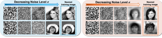
Figure 2. Sampling with Mem./Gen. ReLU DAEs. Left: sampling with a set of memorized ReLU DAEs produces duplicates of training images. Right: sampling with generalized DAEs produces novel images. Details for training and sampling are provided in Appendix C.1, and single-step denoising results are shown in Appendix B.2.
