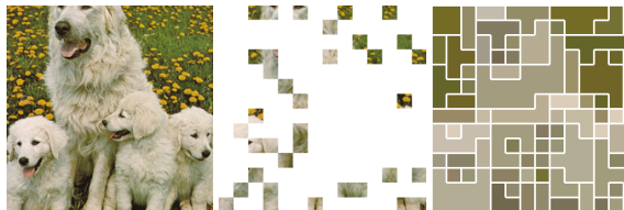
Figure 3. Visualization of token pruning (middle) compared to token merging (right). The visualization shows the remaining tokens after the 10-th layer in ViT-B when pruning or merging 16 tokens per layer.
