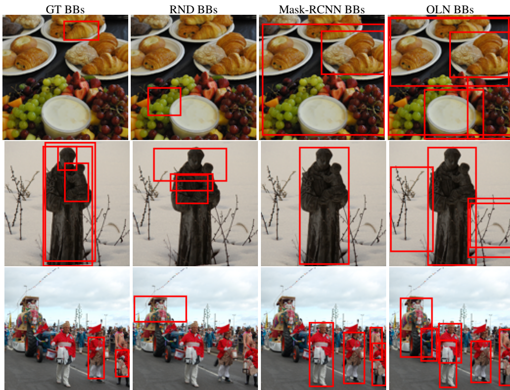
Figure 19: Images from the OpenImages500k ( 128 \times 128 ) dataset split with their corresponding bounding boxes (BBs), overlaid as red rectangles, obtained from either the labeled ground-truth data (GT), sampled as random crops (RND), predicted by Mask-RCNN (He et al., 2017) or OLN (Kim et al., 2022). Discussion in Section G.
