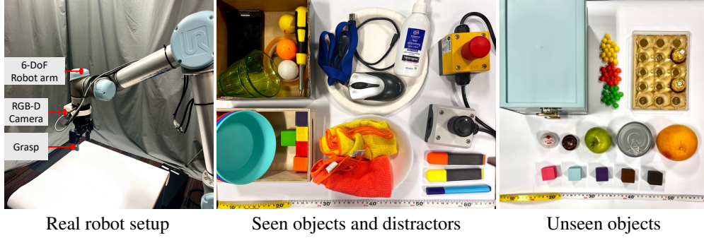
Figure 11: Real robot experiment. The figure shows our physical robot setup along with both seen and unseen objects. Seen and unseen colored blocks are also included.
