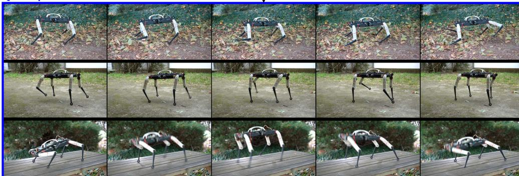
Figure 1: RLWAV trains a video classifier on 8,791 wild animal videos in natural environments to transfer the learned skills to a real quadruped robot with reinforcement learning, without relying on reference trajectories nor hand-designed rewards for each skill. Here, we present the motions resulting from the transfer of the keeping still, walking, and jumping skills to the Solo-12 robot.
