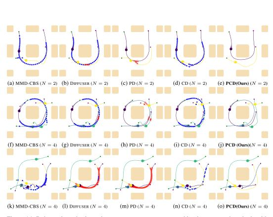
Figure 14: Robot trajectories in environment Highways generated by the compared methods with N=2 and N=4 robots running. Red crosses mark collisions and blue stars mark velocity constraint violations. Each row corresponds to one initial configuration (start and goal positions for each robot).
