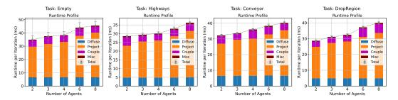
Figure 13: Runtime profile per iteration (in milliseconds) for each task scaling with the number of robots in the multi-robot experiment. The inference batch size for *each robot* is set to 32 and the total diffusion time step is set to 25 for profiling. Results are averaged over 50 random initial configurations for each task and the standard deviations are plotted with error bars.
