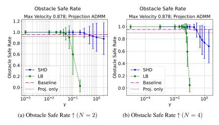
Figure 20: Obstacle safe rates for the coupling strength ablation of **PCD** on task **Highways** with velocity limit  $v_{\rm max}=0.878$ . The obstacle safe rate is defined as the average of an indicator of whether all trajectories are *not* colliding into static obstacles.
