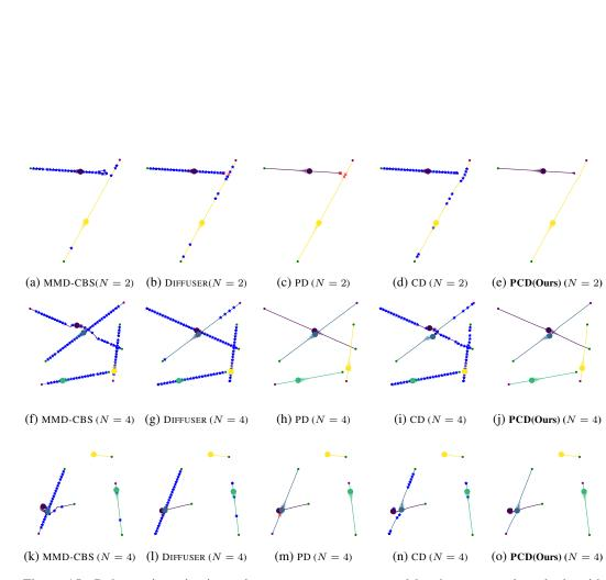
Figure 15: Robot trajectories in environment  ${\tt Empty}$  generated by the compared methods with N=2 and N=4 robots running. Red crosses mark collisions and blue stars mark velocity constraint violations. Each row corresponds to one initial configuration.
