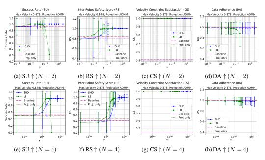
Figure 19: Coupling Strength Ablation of **PCD** on task **Highways** with velocity limit  $v_{\text{max}} = 0.878$ . (a,b,c,d) N = 2 robots; (e,f,g,h) N = 4 robots.
