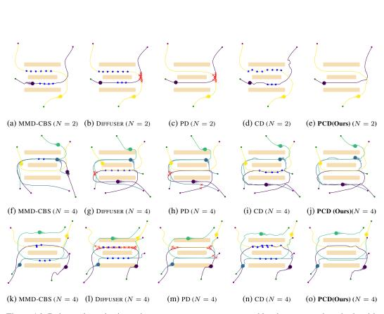
Figure 16: Robot trajectories in environment Conveyor generated by the compared methods with N=2 and N=4 robots running. Red crosses mark collisions and blue stars mark velocity constraint violations. Each row corresponds to one initial configuration.
