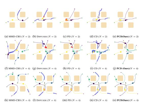
Figure 17: Robot trajectories in environment DropRegion generated by the compared methods with N=2 and N=4 robots running. Red crosses mark collisions and blue stars mark velocity constraint violations. Each row corresponds to one initial configuration.
