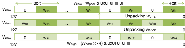
Figure 17. QServe exploits register-level parallelism to significantly reduce the number of required logical operations in UINT4 to UINT8 weight unpacking. channel salience, and then reorder channels so that channels with similar salience are in the same quantization group.
