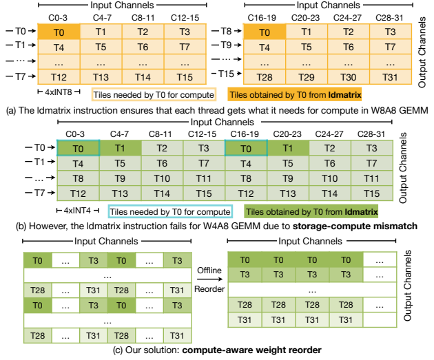
Figure 9. QServe applies compute-aware weight reorder to minimize the pointer arithmetics in W4A8 GEMM main loop.
