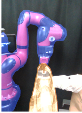
Figure 6: Robot (blue) and garment (orange) segmentation masks after dilation.
