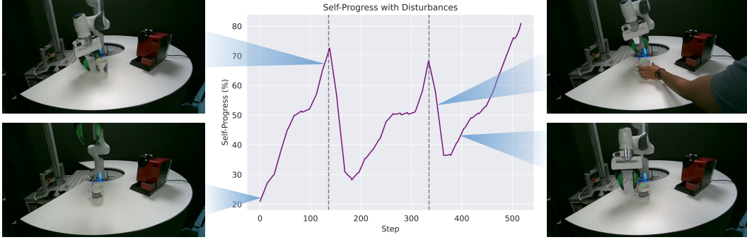
Figure 14: Self-Progress Behaviour with Disturbances. Predicted progress over the course of a task exposed to two different disturbances and resets mid-execution. The task requires the robot to rotate a coffee mug and then grasp it. We indicate the start of the two disturbances where we reset this rotation by the grey dotted vertical lines in the plot.
