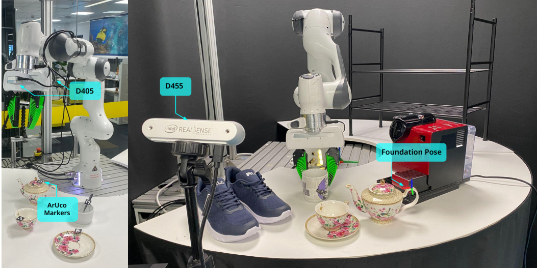
Figure 13: Experimental Setup. Left: Marker-based setup using 2 wrist-mounted D405 Intel Realsense cameras for top down detection. Right: Marker-free setup using a front-facing D455 Intel Realsense camera running Foundation Pose.
