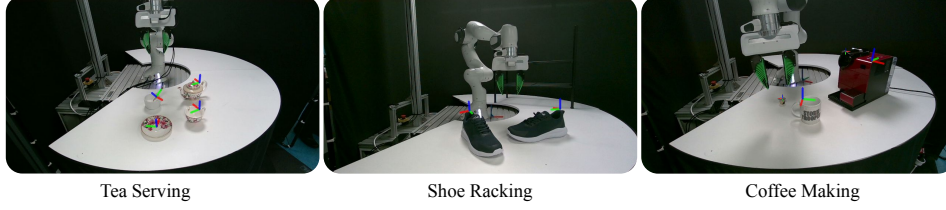
Figure 12: Demonstrating our system across three diverse real-world tasks. The Tea Serving and Coffee Making tasks are very complex compared to many tasks typically encountered in the literature and require multiple sequential object interactions and a high level of interaction precision, e.g. when operating the coffee machine or pouring tea into the cup. Videos of the robot autonomously executing learned policies for all tasks are provided in the supplementary material.
