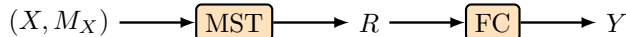
Figure 3: Synthetic data classification pipeline. A multiset sample (X, M_X) is processed by a Multiset Transformer (MST) to generate its representation R . This representation is then used by a fully connected (FC) classifier to make predictions Y . In the context of problem setup (Section 4), MST corresponds to the representation function f_\theta and FC corresponds to the task-specific function g_\phi .
