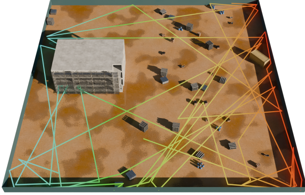
Figure 8. Modified random walk trajectory. We show the trajectory computed by our modified random walk strategy for 500 steps on a procedural construction site scene with seed 0. The camera moves forwards until it reaches an obstacle, in which case it performs a random rotation.
