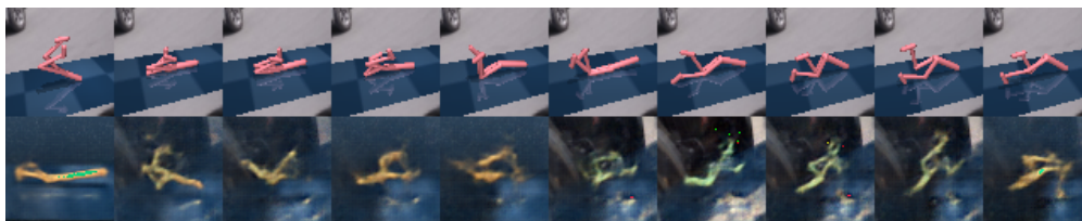
Figure 9: Bottom row shows the reconstruction of a distracted random episode (on the top row) using an RSSM trained on a mixture of two differently distracted environments. We can see that the reconstructed states are split between the two modes of the data and the reconstruction switches robot color and background midway.
