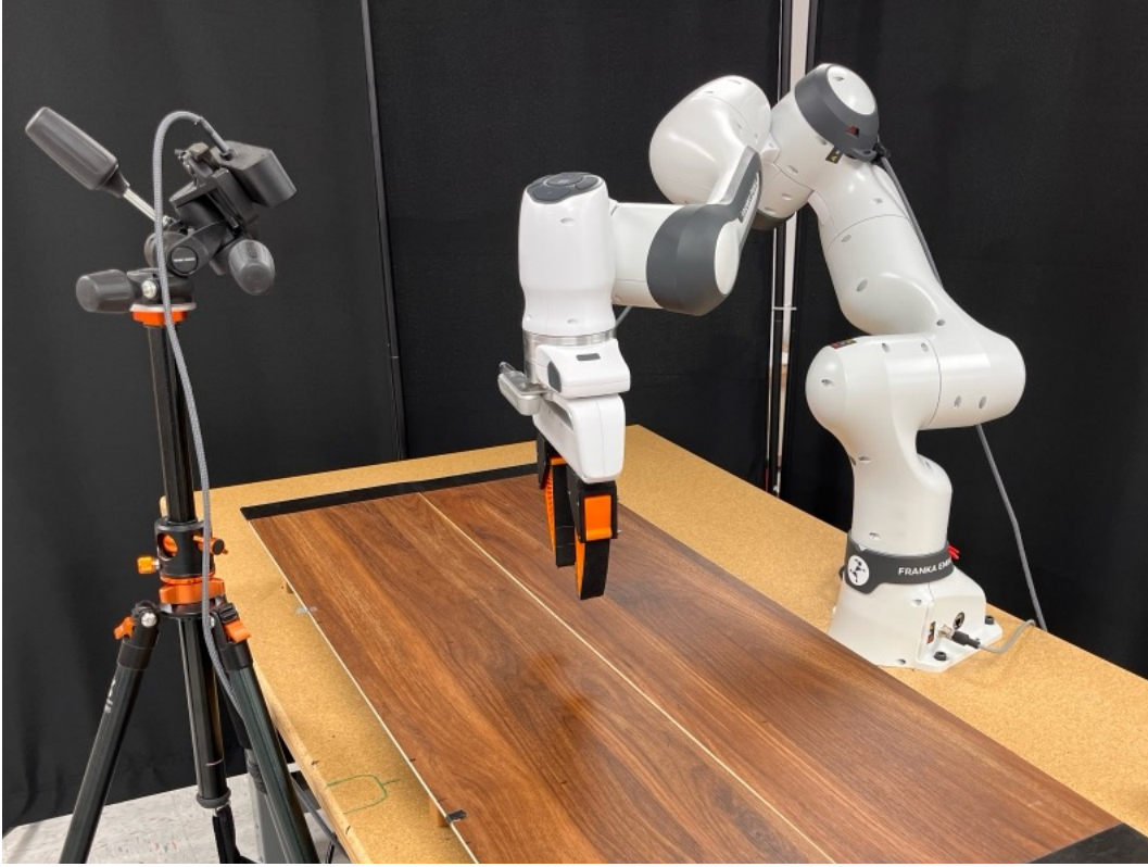
Figure 6: Our hardware experiment setup, we use a Franka Research 3 robot, with a UMI gripper. The RealSense D435 wrist camera, and Zed mini 2i third person camera are placed as shown.
