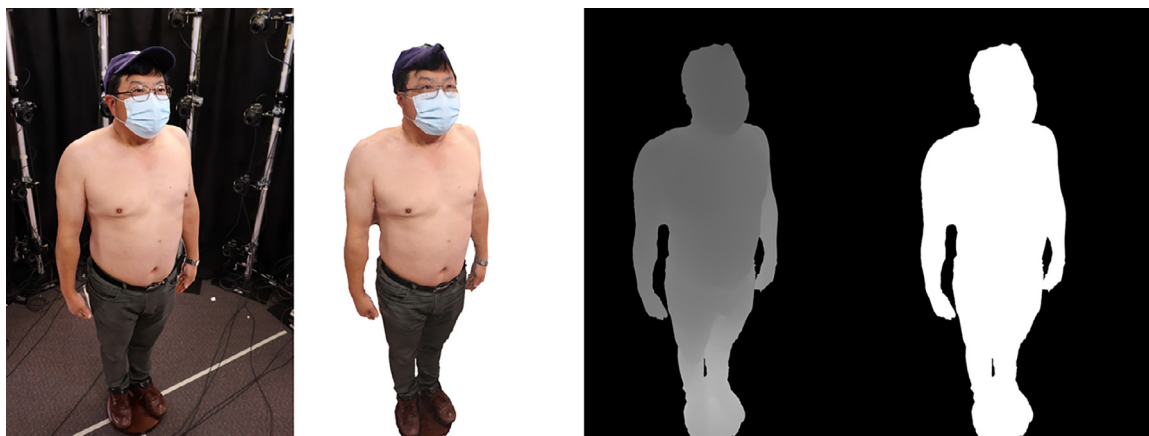
Fig. 12. The input view of preprocessor (left), rendered 3D mesh (middle left), depth image (middle right) and subject mask (right).
