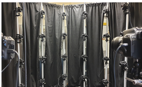
Fig. 3. Whole body photography structure. Camera cage which consist of 15 poles arranged in a cylindrical configuration, each pole with 4 cameras Canon EOS 200D.
