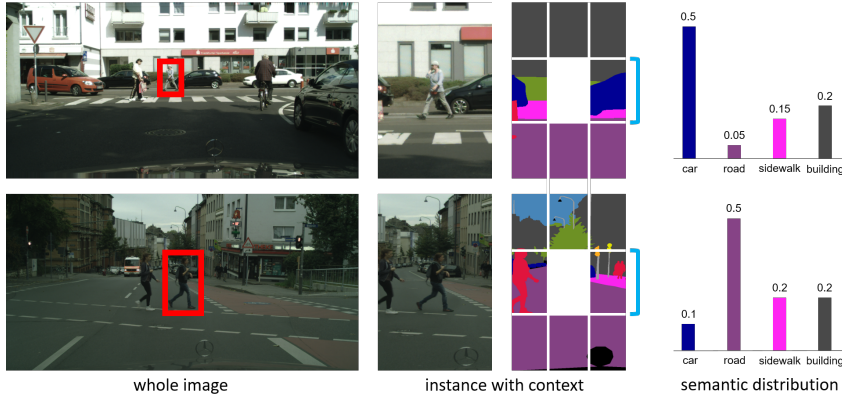
Figure 3: Illustration for evaluating the context similarity between two instances by comparing their semantic distributions in 8 extended regions. From left to right: whole image, instance of interest, semantic distribution of the middle right extended region. We calculate the symmetric KL-divergence between semantic distributions from corresponding regions as the context error.
