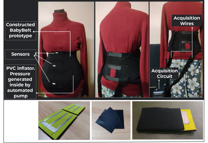
Fig. 6. BabyBelt Prototype. Top image: Left: Front view, Middle: Back view, Right: Circuit integration. Bottom image: Left: Conduction pathway in sensor, Middle: Velostat sheets, Right: Individual Sensor.
