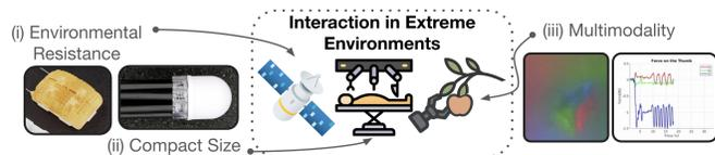
Fig. 1. Mechanically intelligent tactile sensor designs enable contact-rich interaction in extreme environments, from space to surgery to agriculture. Inset are tactile sensor designs towards those application areas: (i) FBG-based tactile sensor with inherent environmental resistance in space; (ii) fiber-based tactile sensor that achieves a compact size for endoscopic procedures; and (iii) multimodal output of visual-capacitive sensor for agricultural robotics.
