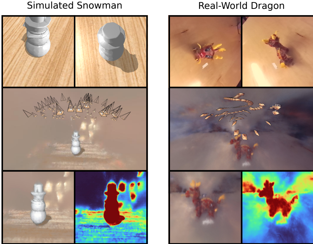
Figure 10: Comparison between NeRFs trained on simulated snowman data and real-world dragon data. This demonstrates the qualitative similarity between the two NeRFs. First row: two of the RGB images used for NeRF training. Second row: Camera poses used for NeRF training. Third row: NeRF-rendered RGB image and accumulation image.
