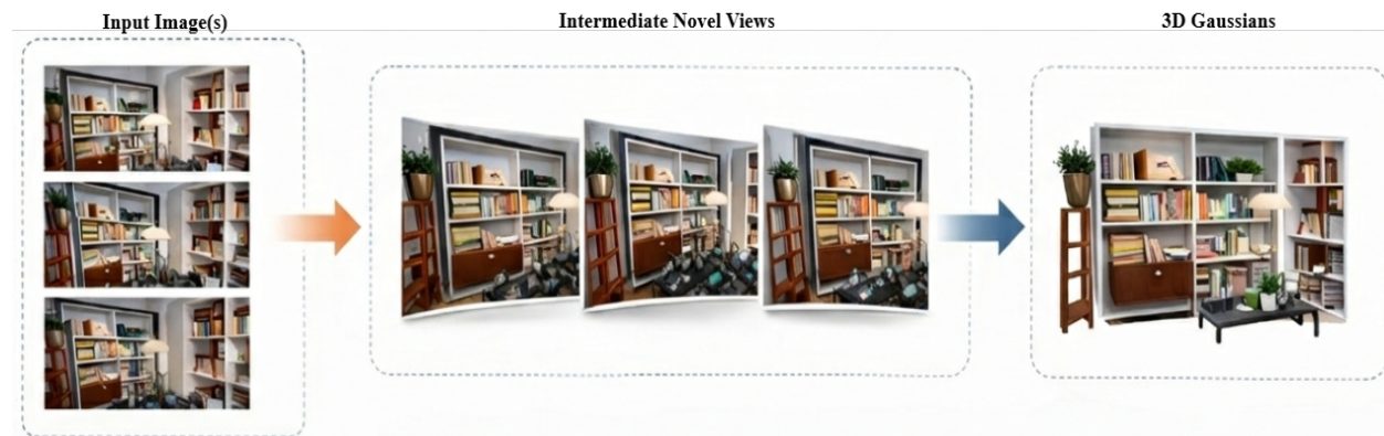
Figure 1: Model Overview: Given one or more sparse input views, the model generates multi-view images and transforms them into a 3D Gaussian representation.
