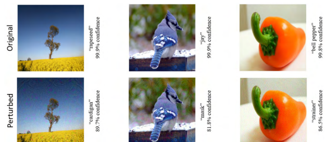
Figure 1: An example of the effect of adversarial attacks on the image classification neural networks taken from Akhtar and Mian (2018). Top: original images which are correctly classified by the neural network with very high levels of confidence. Bottom: same images as above but with small engineered perturbations added to them so that the network now misclassifies them with high levels of confidence.
