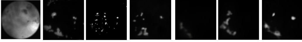
Figure 8: Example of reconstruction results with corresponding SSIM and PSNR values. From left to right: response y , target x , OMP \{0.325, 63.071dB\} , U-Net \{0.636, 66.712dB\} , TransUnet \{0.553, 66.351dB\} , Restormer \{0.625, 66.583dB\} , and TRUST \{0.671, 68.276dB\}
