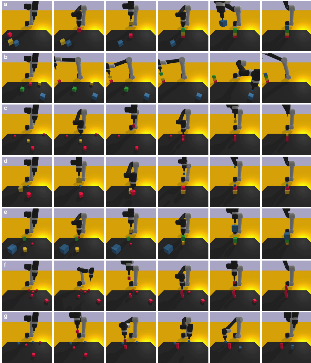
Figure S3: Snapshots of the “stack blocks” task and its variations under user-guided lifelong learning. (a) Stack 4 blocks corner-to-corner at the workspace center. (b) Stack 4 blocks with a 45^\circ rotation at the back-right table corner. (c) Stack blocks by color, with the yellow block on top. (d) Stack blocks from largest to smallest. (e) Stack blocks from smallest to largest. (f) Stack blocks into a zigzag tower. (g) Build two towers sorted by color.
