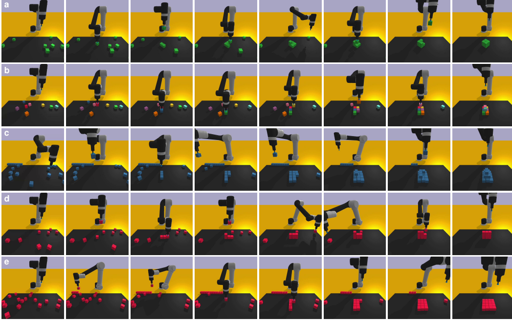
Figure S5: Snapshots of the task “build \{i * j * k\} {structure}”. (a) Build a 2 \times 2 \times 2 cube. (b) Build a 3 \times 2 \times 2 pyramid. (c) Build a 4 \times 3 \times 3 pyramid. (d) Build a 1 \times 3 \times 3 wall. (e) Build a 4 \times 4 \times 1 base.
