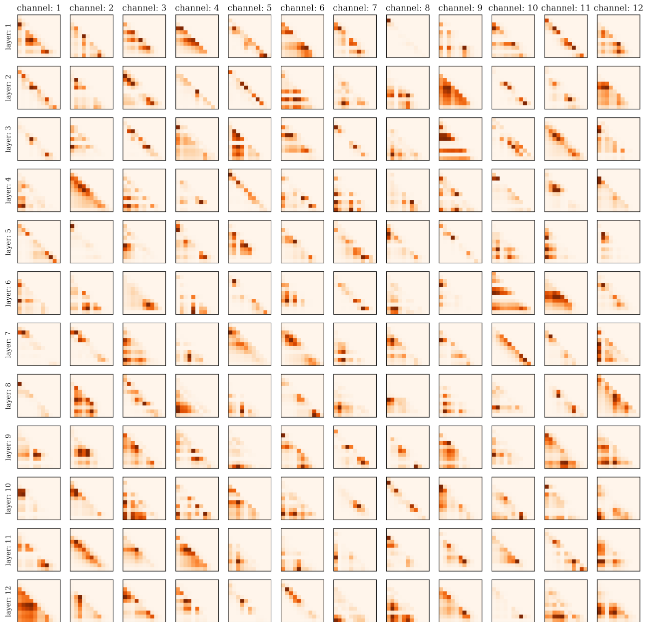
Figure 9. Hyena matrices from a Hyena small (same model used for SuperGLUE downstream evaluations). "We use the test string "Attention is all you need. Attention is". We note that Hyena has a different data-controlled matrix for each channel i.e. for each dimension in its width, since it does not use heads.
